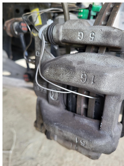
Figure 5. Thermocouples installed to acquire temperatures of disc and brake pad.
